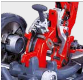
Automatic die head with integrated oil supply
